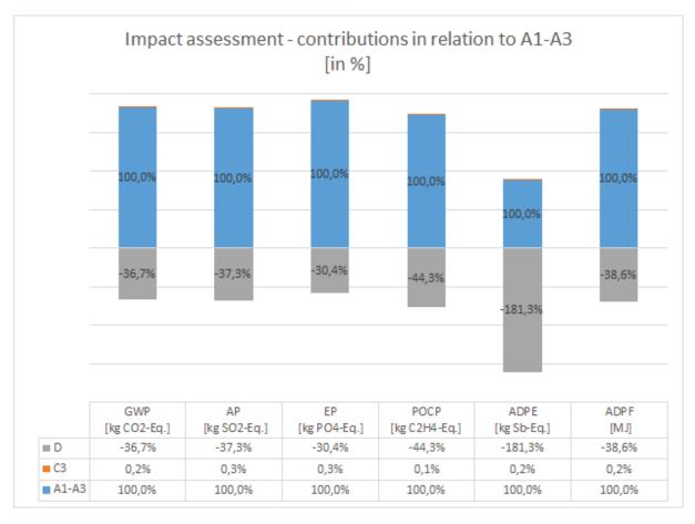
For most categories, the results for product stage (A1-3) contributes with the highest shares. Overall, C3 has a minimized contribution. The credits in Module D have a considerable share, due to the recycling and reuse rate.
